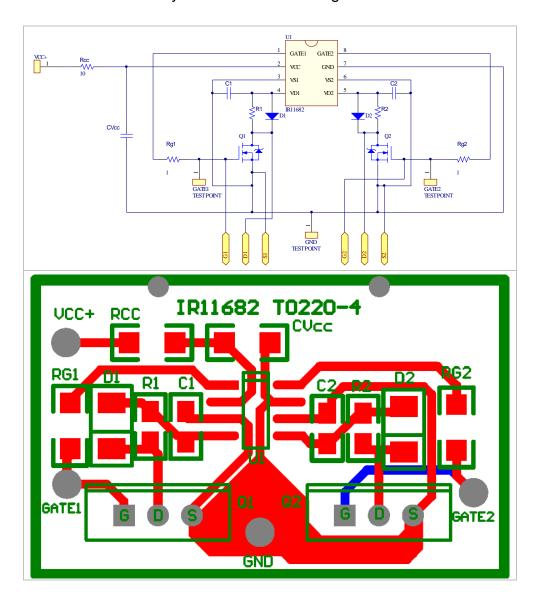
The daughter card shown above is designed to allow easy retrofit in existing systems with minimal system changes. The RCD network that connected to VD pin can be used to adjust the turn-on and turn-off delay of IR11682. If not used, please short R1 and R2  $(0\Omega)$  and leave C1 and C2 open.
