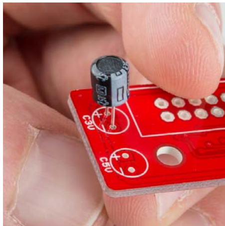
Capacitor Polarity
