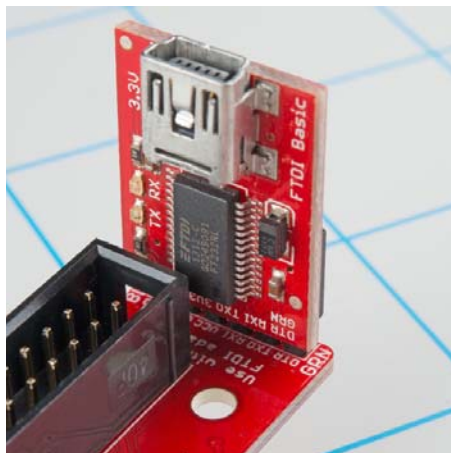
Proper FTDI-basic orientation
