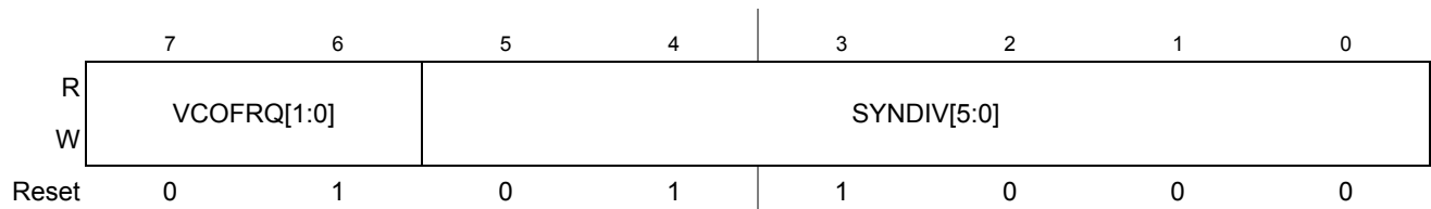
Figure 8-7. S12CPMU_UHV_V11 Synthesizer Register (CPMUSYNR)
