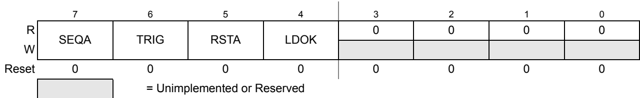
Figure 9-9. ADC Conversion Flow Control Register (ADCFLWCTL)
