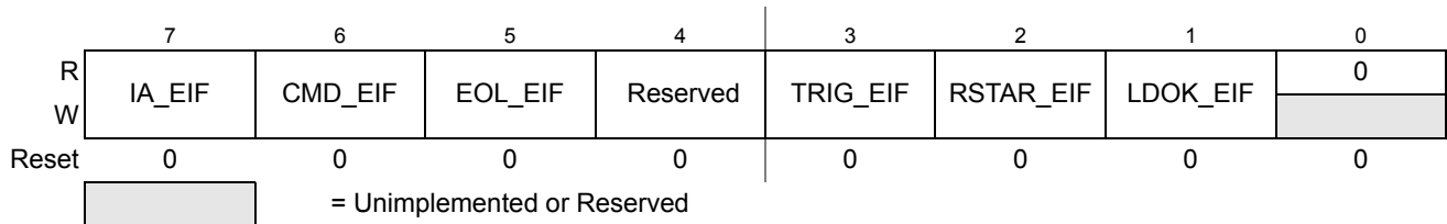
Figure 9-12. ADC Error Interrupt Flag Register (ADCEIF)
