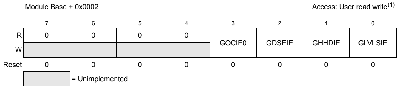
Figure 18-5. GDU2PH Interrupt Enable Register (GDUIE)
