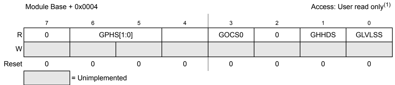
Figure 18-7. GDU2PH Status Register (GDUSTAT)
