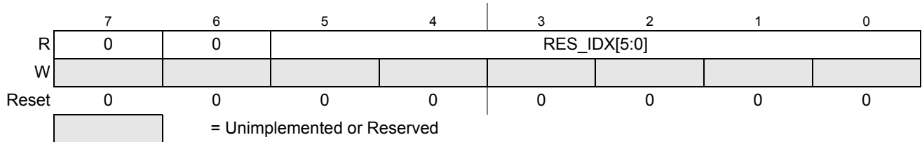
Figure 9-24. ADC Result Index Register (ADCRIDX)
