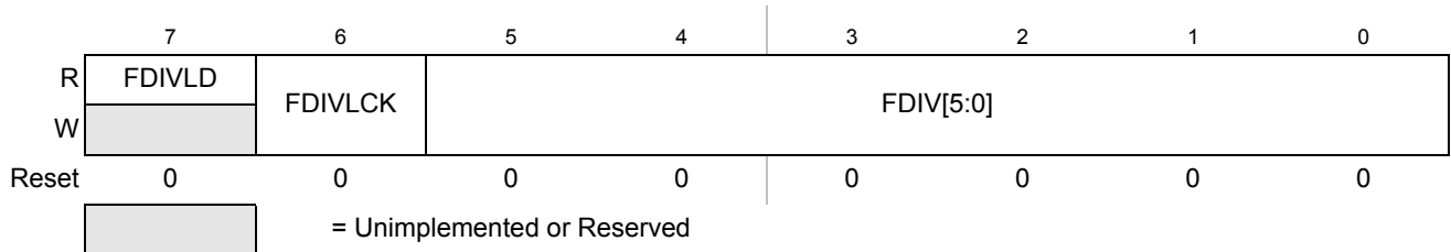
Figure 19-5. Flash Clock Divider Register (FCLKDIV)
